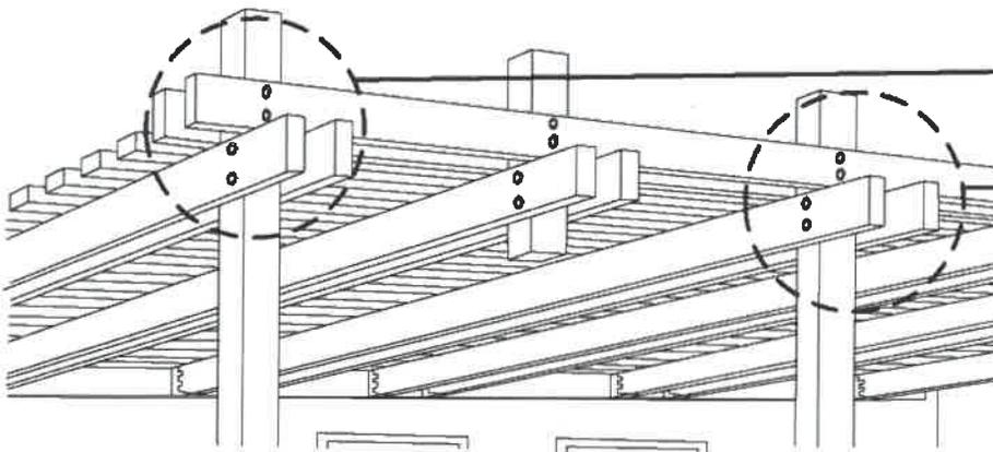
**NOTE:** KNEE BRACING REQUIRED WHEN RAFTER SPAN EXCEEDS 12 FEET
